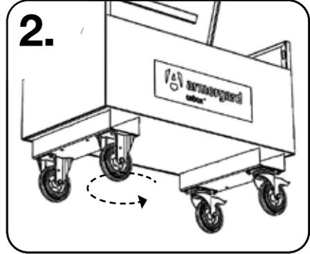
2. Repeat for the other 3 wheels. Once complete, check all nuts are tight, and then ensure the two braked castors can swivel 360° before lowering the OxBox.
