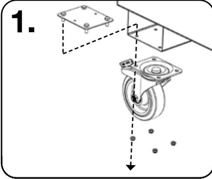
1. Only the OX3 and OX4 can be fitted with castors. Lift the box onto a stable platform, and then insert castor plates into the forklift skids. Put the castor wheel in place and use a 13mm socket to tighten the M8 nylocks.
