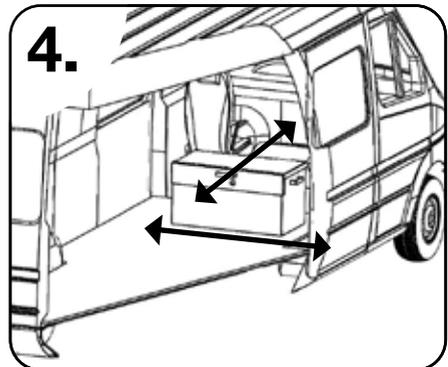
Once installed, test by pulling and pushing the box vigorously in various directions. Bear in mind that an empty box can more than triple its weight in the event of an emergency stop, so it is imperative to ensure it is firmly fixed down.
