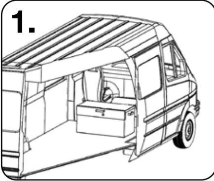
To install an OxBox in a vehicle, these instructions **MUST** be followed. The van boxes come with coach bolt holes predrilled in the floor of the box for fixing them down.
