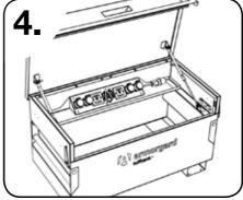
The shelf should now drop into place - depending on the model this will either be on the lugs provided or onto the shelf created by the recessed handles.
