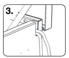
Up to 2 cables can be fitted into the cable pass-through, so a power supply and a tool can be fitted through simultaneously. The lid can then be closed and locked for secure charging.
