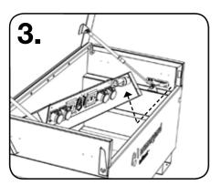
Slot the right hand side of the shelf down in front of the gas strut, bring it underneath, and back up behind the gas strut.
