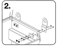
Thread the M10 coach bolts through the lifting eyes, then through the box. Inside the box add a backing plate, M10 washers and nylocks to each bolt as shown.
