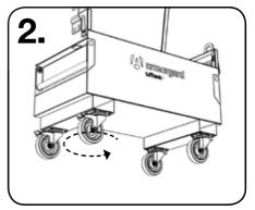
Repeat for the other 3 wheels. Once complete, Check all nuts are tight, and then ensure the two braked castors can swivel through 360° before lowering the TuffBank.
