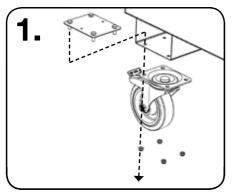
All TuffBanks except TB1 & TB12 can be fitted with castors. Lift the box onto a stable platform, and then insert castor plates into the forklift skids. Put the castor wheel in place and use a 13mm socket to tighten the M8 nylocks.
