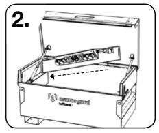
Slide the left end of the shelf into the TuffBank, under the gas strut with the SlamStop safety stay.
