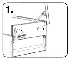
All TuffBanks except TB1, TB12 & TB21 can be fitted with crane lifting eyes. To fit the kit, use a 10mm metal drill bit to drill out the 4 pilot holes located on each side of your TuffBank.
