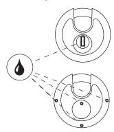
Insert the key and open and close the lock multiple times to ensure the lock is working freely. Re-attach the disc lock and the lock housing using the 2 M8 nuts.
