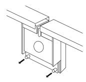
2 Locate the keyhole and the 4 holes on the back of the disc lock and blow all dust and dirt out the lock using a compressor or a pressurised canister.
