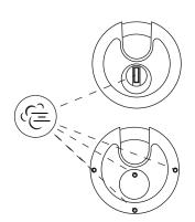
3 Lubricate lightly in the 4 small holes and the key hole. We recommend using a lubricant spray that contains PTFE additives for the best performance.
