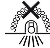
Luminaires not suitable for covering with thermally insulating material
