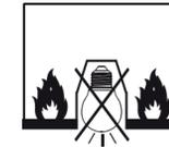
Luminaires are only suitable for mounting on non-combustible surfaces
