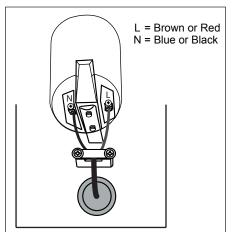
Having correctly identified the wiring from your existing light fitting, pull the wire through the hole and connect to the lampholder inside the product in the following way:
