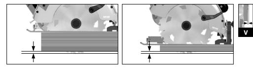
Adjust the cutting depth to the thickness of the workpiece. Less than a full tooth of the blade teeth should be visible below the workpiece.
