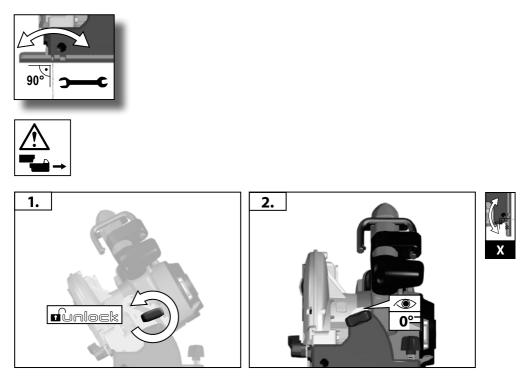
If a correction of the 90° angle of the guide-plate to the saw blade is necessary, use the correction screw.
