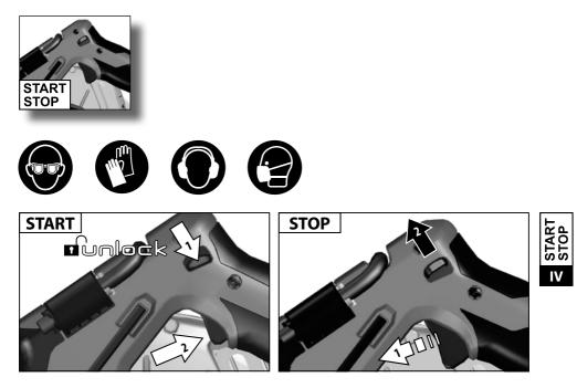
For safety reasons this power tool is fitted with a switch lock and the On-/Off switch cannot be locked in the "On" position
