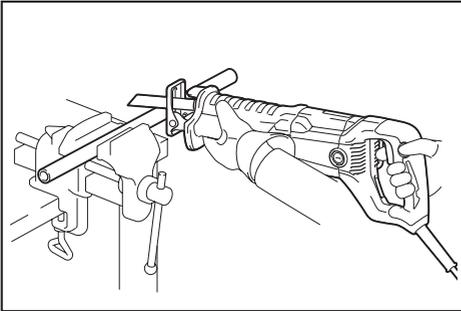
**NOTICE:** Do not cut the workpiece with the shoe away from the workpiece or without the shoe.
