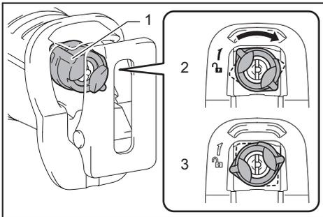
► 1. Blade clamp lever 2. Released position 3. Fixed position
