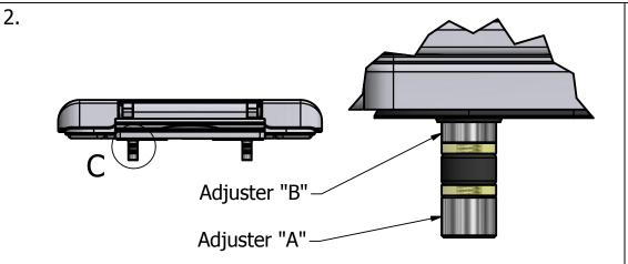
Familiarise yourself with the adjustment points. Adjuster "A" is for hole size changes Adjuster "B" is for hole depth changes
