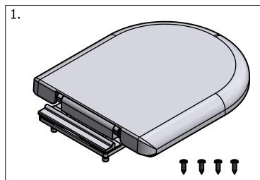
Remove seat from packaging and locate 4x small self tapping screws. Put these safely to one side.
