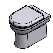
While the lid is clamped down, slide it to your prefered position on the toilet pan. Hold the base of the hinge while opening the handle to reveal the adjuster plates.
