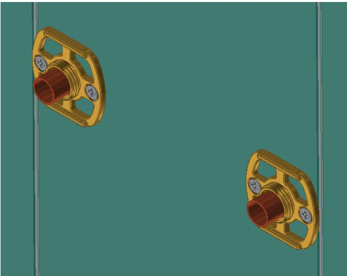
Place the backing plate over the pipe. Drill and screw the backing plate to the wall using a suitable method for your wall. Check for pipes and cables before drilling.
