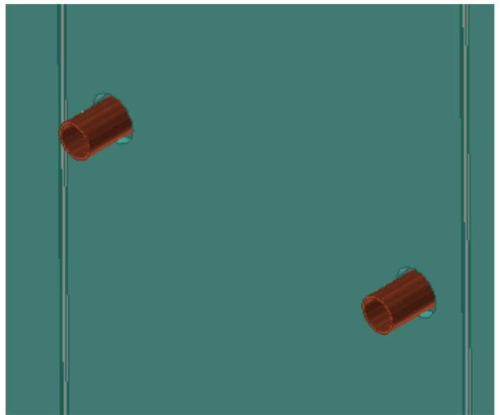
Cut the pipes down leaving 19mm protruding from the face of the wall. Do not leave any sharp edges or burrs on the pipes.
