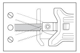
You can use both jig saw blades (B type) and recipro saw blades according to your work. Insert the recipro/ jig saw blade straight into the blade clamp and tighten it by hex wrench. Pull the recipro/jig saw blade lightly to make sure that the recipro/jig saw blade does not fall off during operation.
