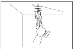
You can use the switch lever or trigger according to your work.
