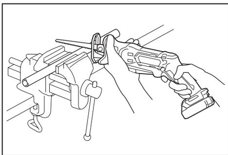
Press the shoe firmly against the workpiece. Do not allow the tool to bounce. Bring the reciprocating saw blade into light contact with the workpiece. First, make a pilot groove using a slower speed. Then use a faster speed to continue cutting.
