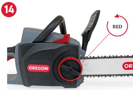
**STEP 14:** Reverse direction of the **RED** chain tensioning ring until you observe the chain loosen slightly.
