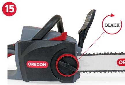
**STEP 15:** Tighten fully the centre **BLACK** side cover release knob.
