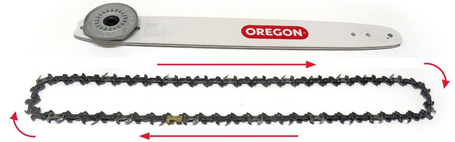
**STEP 7:** To properly install the chain on the guide bar, check that the cutting edges of the teeth go forward.
