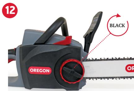
**STEP 12:** Then lightly tighten clockwise the center **BLACK** side cover release knob.
