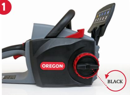
**STEP 1:** Remove the side cover by turning the **BLACK** side cover release knob.
