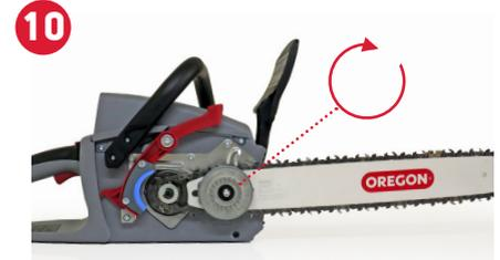
**STEP 10:** Loop the saw chain around the drive sprocket, turn the tensioning gear clockwise to begin tensioning the chain.
