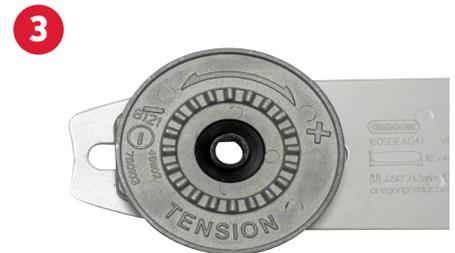
**STEP 3:** Now the tensioning gear has been flipped, make sure the the Oregon logo is the right way up on the bar.
