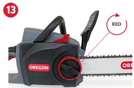
**STEP 13:** Tighten fully the **RED** chain tensioner ring until the lowest cutter underneath the bar solidly contacts the bar.
