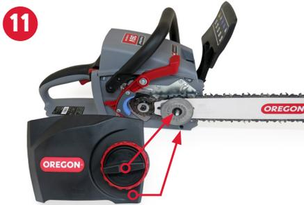
**STEP 11:** Install the side cover, making sure the chain catcher pin is properly seated in its hole, and aligning the tensioner on the side cover with the tensioner on the guide bar.
