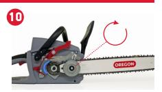
**STEP 10:** Loop the saw chain around the drive sprocket, turn the tensioning gear clockwise to begin tensioning the chain.
