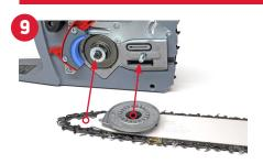
**STEP 9:** Place the guide bar on the bar pad, inserting the hole of the tensioning gear in the bar stud.
