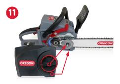
**STEP 11:** Install the side cover, making sure the chain catcher pin is properly seated in its hole, and aligning the tensioner on the side cover with the tensioner on the guide bar.
