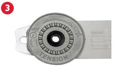
**STEP 3:** Now the tensioning gear has been flipped, make sure the the Oregon logo is the right way up on the bar.
