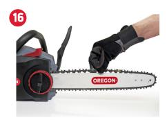
**STEP 16:** Check the tensioner by pulling on the chain and observe the "snap" of the chain when released.
