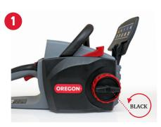
**STEP 1:** Remove the side cover by turning the **BLACK** side cover release knob.
