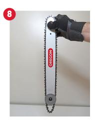
**STEP 8:** Grab the nose of the bar and feed the chain into the groove of the bar.
