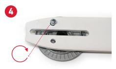
**STEP 4:** Turn the bar over, insert and properly tighten the screw from the back side of the chain tensioning gear to attach it onto the guide bar.
