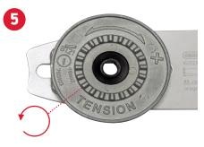
**STEP 5:** Turn the tensioning gear anti clockwise as far as it will go to fully loosen the chain.
