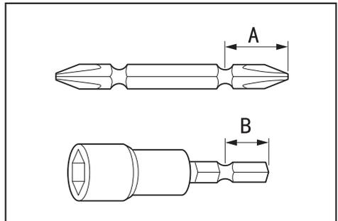
Use only driver bit/socket bit that has inserting portion shown in the figure. Do not use any other driver bit/socket bit.
