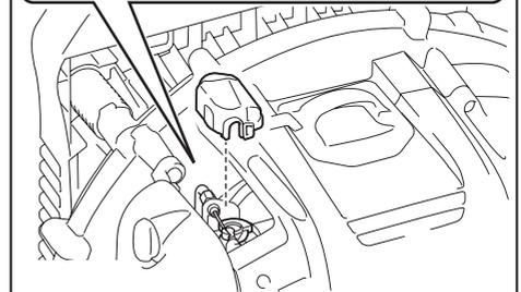
► 1. Throttle valve 2. Idling adjusting screw 3. Control cable 4. Throttle valve stopper
