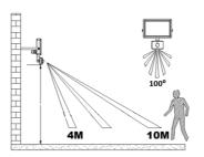
Mounting the light at excessive height may reduce the performance of the PIR.
