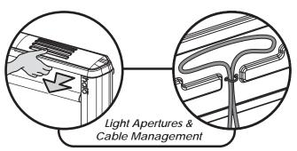
To maximise the effectiveness of **Halo** in catching flying insects, the top of the product has light apertures to increase the UV irradiance emitted from the product. However, these apertures can be covered to protect the glueboard from debris and prolong its life, by simply sliding the reflective aluminium cover forward.
