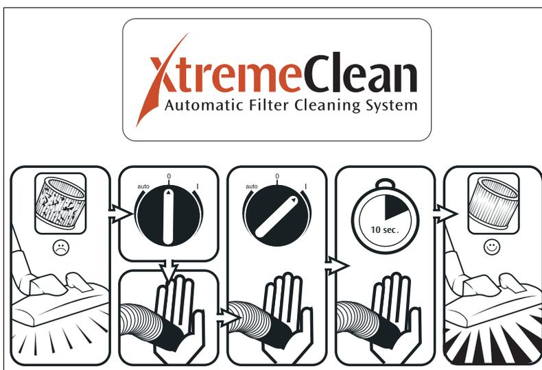
To ensure that suction performance is always at its best, the filter element is automatically cleaned during operation. We recommend complete cleaning if the filter element becomes extremely dirty.
