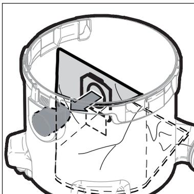
4. Press the filter bag connection firmly on to the inlet fitting.
