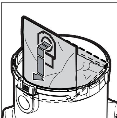
3. Insert the filter bag into the dirt tank.
