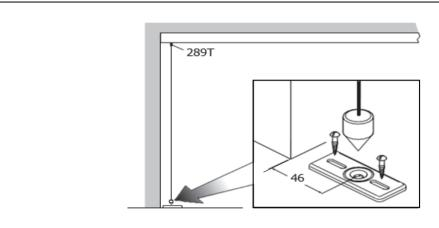
**STEP 11** i) For HF25 kits, please skip to step 13. For HF40 kits, cut guide channel to required length. ii) Use a plum line to align the guide channel with the track, mark out positioning with a pencil ready for routing
