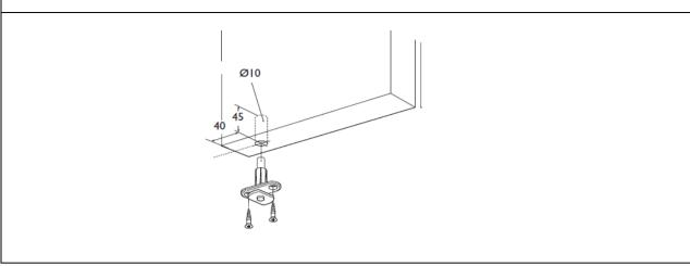
STEP 5: Attach guide to bottom of the doors (HF40 kits only)
