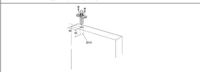
STEP 3: Fit hangers to doors - for 2 door applications fit hanger to 2nd door. For 4 door applications, fit hangers to 2nd and 4th doors.
