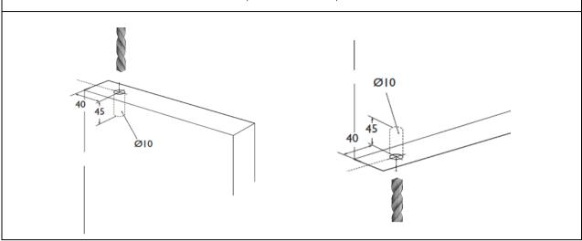
STEP 2: Position and secure top pivot body to the top of the pivot door
