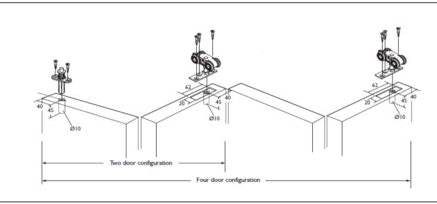
STEP 4: Position and secure the bottom pivot body to the bottom of the pivot door.
