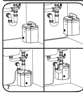
The boiler unit can be free standing or mounted on the wall inside the cupboard. points to consider :
