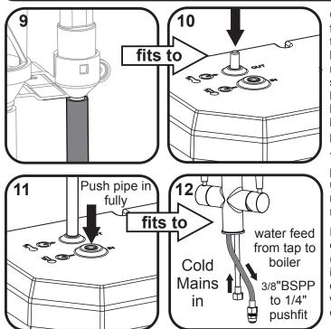
Connect the hot tube from the drain valve to the hot outlet of boiler. The pipe needs to be a smooth run with no kinks or sharp bends, the tube can be cut to suit your particular installation.
