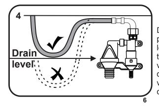
The drain valve needs to be fitted as high as possible, this is to help prevent the possibility of a blocked sink flowing out of the drain valve.
