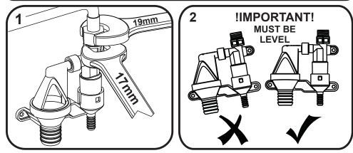
Connect drain valve assembly to the open hot delivery pipe of the tap. You may wish to leave this connection loose until the final position of the valve is known.
