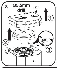
If the boiler is being mounted on the wall lift off the cover complete with knob (1) and the insulation cap (2) to expose the mounting holes (3).
