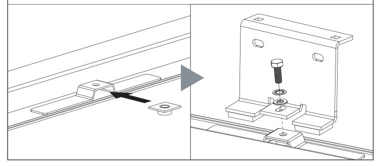
Place roof bars onto the roof brackets with the t-slot facing upwards, secure using top hat brackets, M6x16 coach bolts & M6 serrated nuts.
