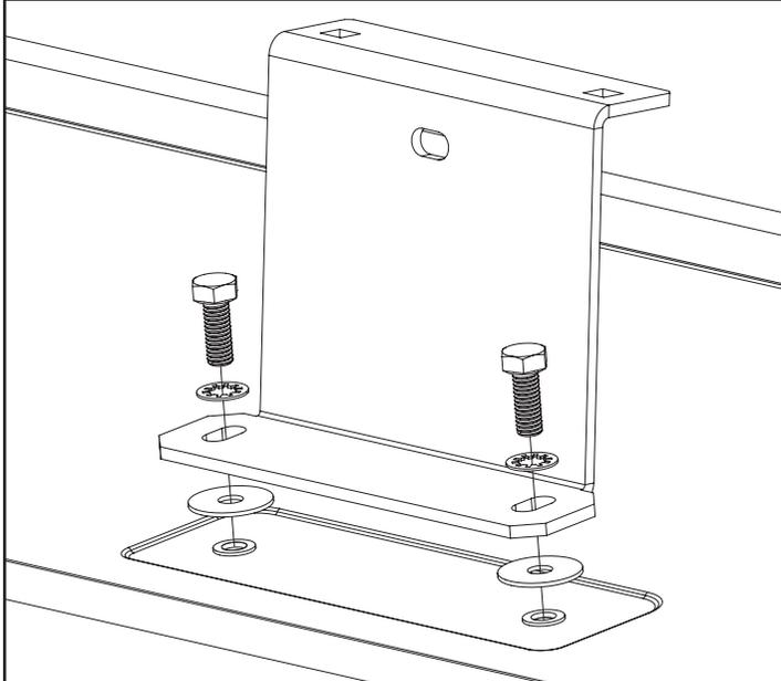
**4** Place roof bars onto the roof brackets with the t-slot facing upwards, secure using top hat brackets, M6x16 coach bolts & M6 serrated nuts.
