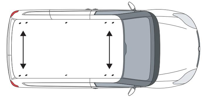
**3** Secure roof brackets to the vehicles fixing points using M6x16 hex bolts, M6 shakeproofs & rubber washers. Ensure that the top hat flange is facing inwards.
