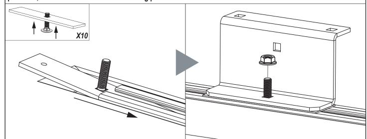
Place roof bars onto the roof brackets with the t-slot facing upwards, secure using top hat brackets, M6x16 coach bolts & M6 serrated nuts.
