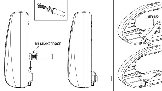
Assemble the roller spigot, M8x20 hex bolt and M8 shakeproof washer together. Place the assembly into the roller. Slide the roller onto the spigot fitted in step 10 and drop the other end into position. Tighten using the supplied tool (ME0182).
