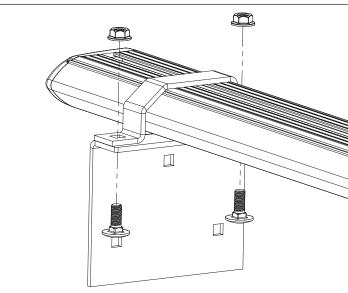
Place assembled roof bars onto the vehicles roof and clamp the roof brackets to the vehicles side rail using M6x25 coach bolts, fixing brackets & M6 serrated nuts.
