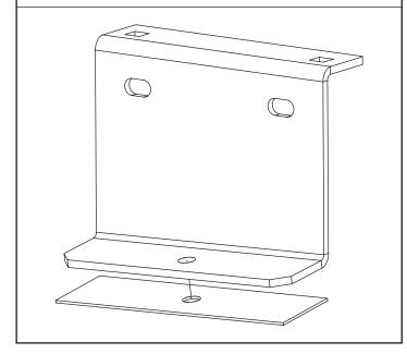
Secure the rear and middle roof brackets by bolting through the vehicles fixing points using M6x30 hex bolts, M6x20 washers & rubber washers. Secure under the roof using M6x25 washers & M6 serrated nuts. Ensure that the top hat flange is facing inwards.
