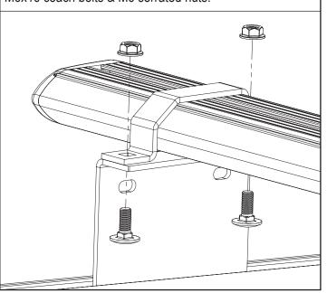
Flex the top hat covers over the top hat brackets into position as shown below. Ensure that the covers click into the front and rear of the top hat brackets.
