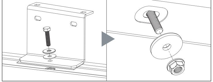
Secure the front roof brackets by **carefully** loosening the edge of the roof liner enough to hold the front fixing point tool up to the fixing point. Once in position bolt down through the fixing point, into the bush using M6x30 hex bolts, M6 shakeproofs, M6x20 washers, & rubber washers. Ensure that the top hat flange is facing inwards.
