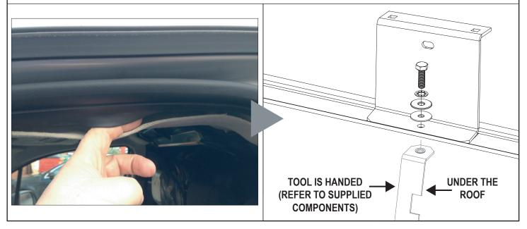
Place roof bars onto the roof brackets with the t-slot facing upwards, secure using top hat brackets,
