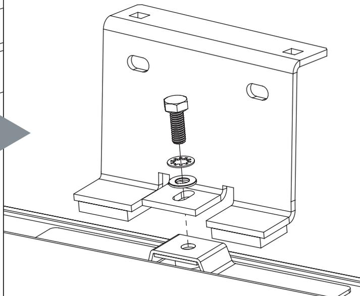
**4** Place roof bars onto the roof brackets with the t-slot facing upwards, secure using top hat brackets, M6x16 coach bolts & M6 serrated nuts.
