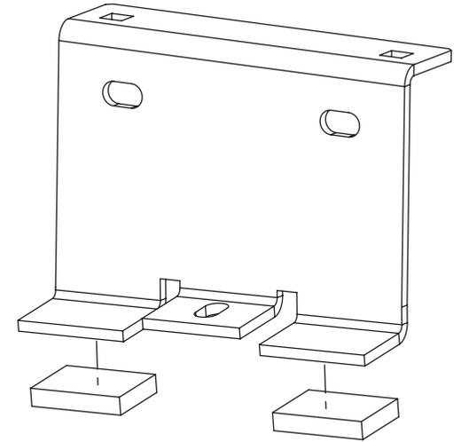
**3** Secure roof brackets to the vehicles fixing points by placing the roof bracket plates under the fixing points and secure using M6x16 hex bolts, M6 shakeproofs & M6 washers. Ensure that the top hat flange is facing inwards.
