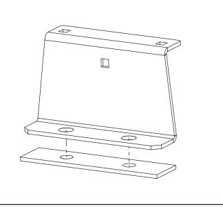
Remove roof plugs to reveal the vehicles fixing points. Secure roof brackets by bolting through the fixing points using M10x35 hex bolts, M10 washers & rubber washers, secure under the roof using M10 serrated nuts. Ensure that the top hat flange is facing inwards.
