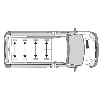
Secure roof brackets to the vehicles fixing points using M6x10 hex bolts & M6 shakeproofs. Ensure that the top hat flange is facing inwards.
