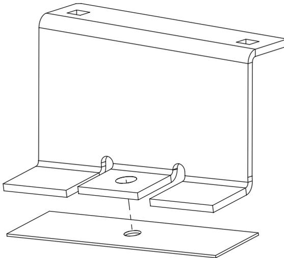
**4** Secure roof brackets to the vehicles fixing points using M8x20 hex bolts & M8 shakeproofs. Ensure that the top hat flange is facing inwards.
