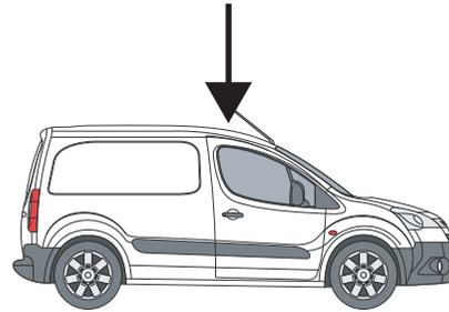
**2** Remove roof plugs to reveal the vehicles fixing points.
