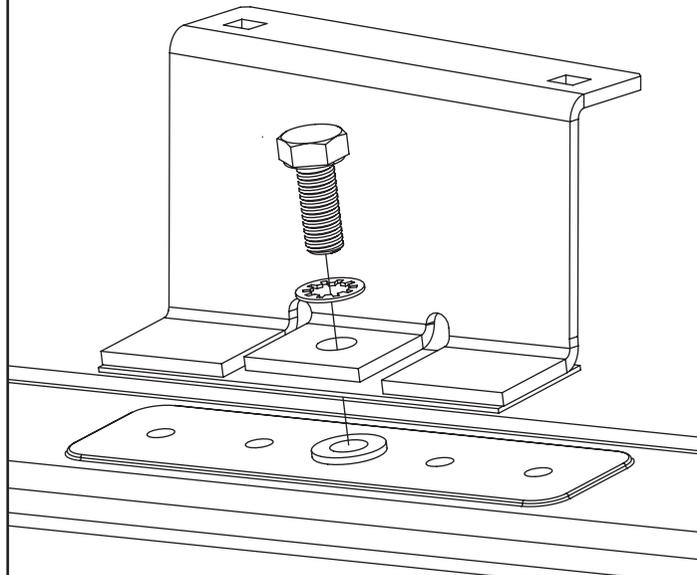
**5** Place roof bars onto the roof brackets with the t-slot facing upwards, secure using top hat brackets, M6x16 coach bolts & M6 serrated nuts.
