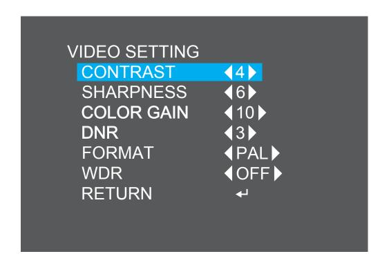
**Format (PAL-NTSC):** The reason for this option is mainly for indoor mounted cameras. Artificial lighting flickers slightly at the frequency of mains power which the cameras are able to see and shows on your screen as a flickering image. The correct setting here will eliminate any flicker produced by artificial lighting. For USA and Canada select NTSC, for AU, UK and most of Europe select PAL.
