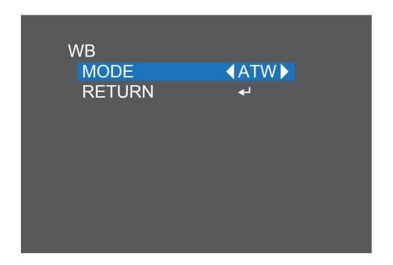
**ATW (Automatic White Balance):** The camera sets the White Balance according to the light it receives. We recommend you use this setting in most circumstances.
