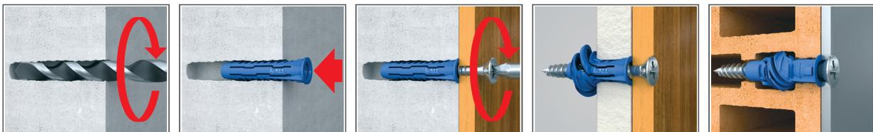
1. Drill a hole of required diameter.
