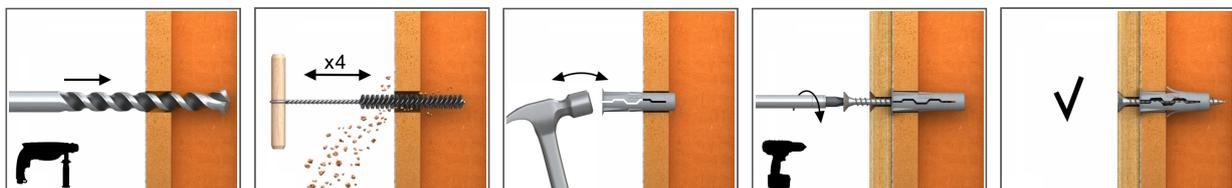
1. Drill a hole of required diameter.
