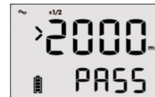
Displaying result of 1st ½x test (Figure.5)
