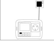
Connect the Instrument to the mains supply using the mains plug test lead (for mains powered leakage and RCD testing)
