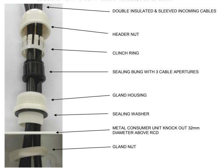
The kit comprises a 32mm insulated cable restraining gland, which is fitted by removing the knockout above the incoming terminals and fixing into position with the nut included. The incoming supply cables must be passed through the 3 aperture sealing bung. The sequence of assembly over cables is as shown above. Tighten the gland and header nut when installation of
