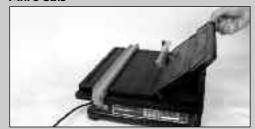
For mitre cuts, raise the hinged section of the table to the required angle (22.5° or 45°)
