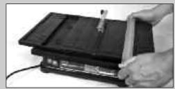
Place the Rip Guide on the table top and line up with the measurement graduations on either edge to the required size. When correctly aligned, tighten the rip guide securing nuts.
