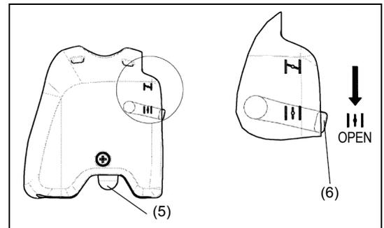
**NOTE:** - If you pull the starter handle repeatedly when the choke lever is in the at "↓" position, the engine will not start easily due to excessive fuel intake.
