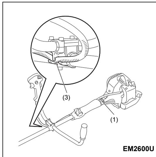
CAUTION: Do not position the throttle cable as shown. Otherwise curved cable may cause high idle speed, and uncontrollable blade may cause personal injury.
