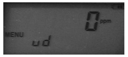
"Oppm ud (ud=under)" will display leaks in steps. The steps are Oppm, ud 500ppm, ud 1000ppm, ud 3000ppm, ud 5000ppm, ud 9999ppm
