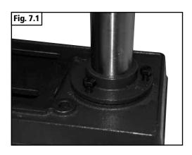
2. Fit the table locking handle in to the table support casting. Locate the table assembly onto the column and secure with the locking handle. (Note that one side of the support casting has a plain bore, and the other side has a tapped hole. Ensure that the locking handle is passed through the plain bore and into the tapped hole in order for the table support casting to clamp correctly around the column) (Fig. 7.2).
