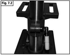
3. Attach the head assembly of the drill to the top of the column and secure using two M8 x 8mm socket head grub screws. Before fully tightening the screws check that the head is correctly aligned with the base so that the spindle is above the centre line of the base casting (Fig. 7.3).
