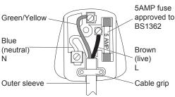
Warning: Never connect live or netutral wires to the earth terminal of the plug. Only fit an approved 5 Amp BS1363/A plug and the correct rated fuse.
