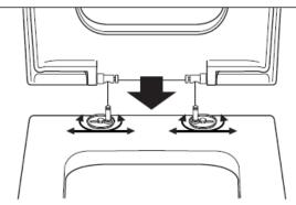
**3.** Lower the seat/cover onto the pan, engaging the hinge pins with the hinge bases. The position of the hinge bases may need to be adjusted to allow this.
