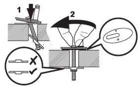
Assemble the hinge and gasket and slide the tab and bolt through the pan until it engages on the underside.
