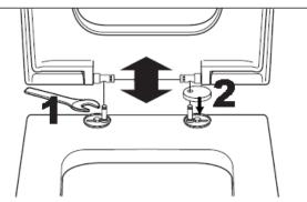
**5.** Once adjusted, remove the seat/cover and tighten the bases with a spanner. Clip the hinge covers in place before replacing the seat/cover. Care should be taken not to overtighten the fixings.
