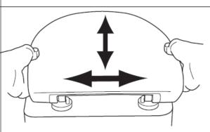
**4.** Adjust the hinges to centralise the seat on the pan and to allow the correct degree of seat/cover overhang at the front
