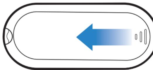
2 Pull out the protective plastic strip to engage the battery and activate the Key Fob.
