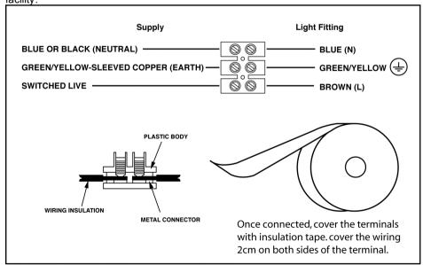
Please note: For new installations, check for any electrical cables or pipe work (gas/water) in the vicinity of the intended mounting point for this product, before proceeding with the installation.
