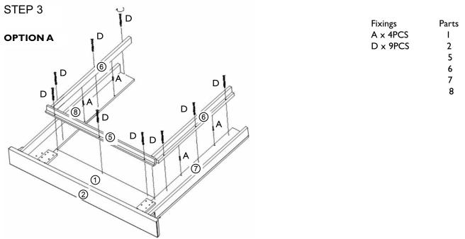
Place the wide inside leg panels (6) on the the back of the legs (7 and 8). Secure the two using 2x dowels (A), glue (E) and 3x wood screws (D) in each side. Now connect the wide inside top (5) to the backboard (I) using 3x wood screws (D).
