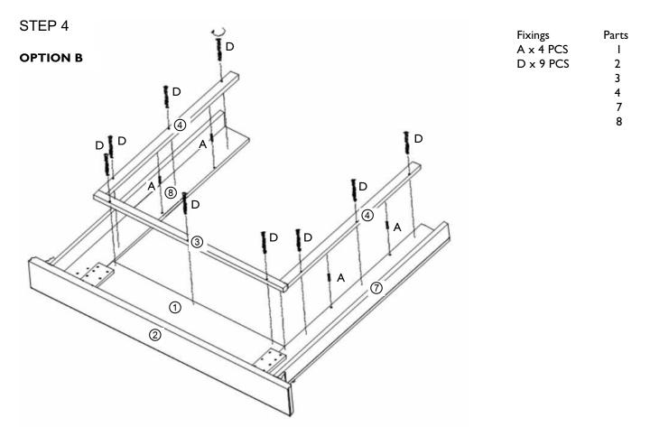
Use the Glue (E) in the dowel holes before inserting 2 dowels (A) into the left and right hand legs (7 and 8). Now put a small amount of glue (E) in the dowel holes of the narrow inside leg panel (4). Push the narrow inside leg panel (4) on to the dowels (A). Use 3x screws (D) on each leg to secure the panel down. Next use 3x woods screws (D) to install the narrow inside top panel (3) to the backboard (1).
