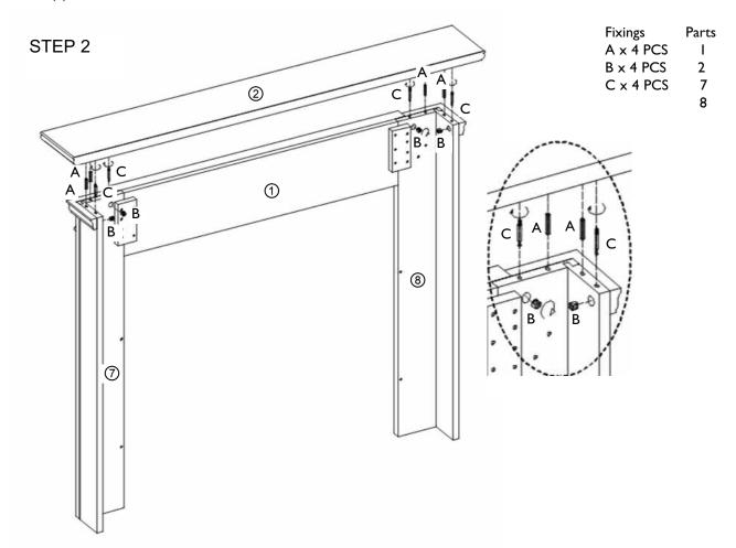
Fit cam locks (B) into side panels (7&8). Using a drop of glue (E) in each dowel hole, insert 2 dowels (A) in to the left leg (8), and repeat on the right leg (7).
