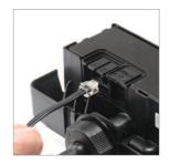
Plug the end of the attached data cable feeding from the splitter box into **port 1** of the Digital Diverter.
