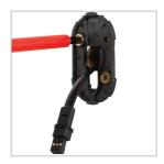
Push the data cable plug into the back of the button fully home to ensure a water tight seal making sure the seal is no longer visible.
