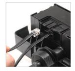
Plug the end of the 10m low voltage data cable feeding from the main controller, as well as the end of the 10m low voltage data cable feeding from the remote button, into the two side by side entry ports on the splitter junction box as shown.
