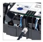
Plug the other end of the 2m data cable (supplied with the Digital Diverter) into port 2 on the Digital Diverter.
