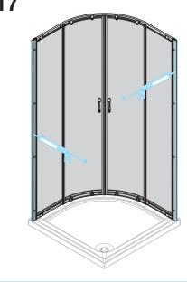
Apply Silicone sealnt, (not supplied) between Wall Channel as shown.
