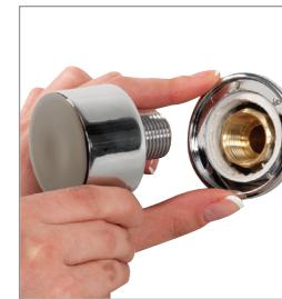
**4** Ensuring the hose washer is in place, connect the hose (supplied separately) to the wall outlet assembly and run the shower for 15 seconds without the handset attached to clear any debris, which may be present.
