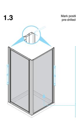
Mark position of pre-drilled Wall Channel
