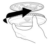
Once the smoke alarm has been fitted onto the mounting plate correctly, the internal power pack will activate. The red LED on the front of the alarm should now flash once every 40 seconds to show that it is active. \*When attaching to some older FireAngel mounting plates, it is only possible for the alarm to be attached in one orientation. Contact the FireAngel Technical Support Team for advice if required (see page 21)
