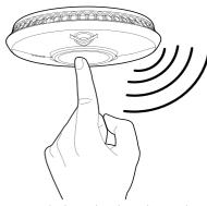
**a** Press and release the silence button, the alarm sound will shortly stop.
