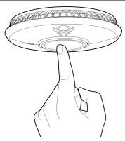
The alarm must be properly attached to the base plate before it can be tested
