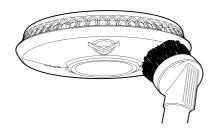
**WARNING:** Your FireAngel smoke alarm may false alarm when it is being cleaned using a vacuum cleaner.
